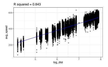
The linear model with log\_dist  $(R^2 = 0.843)$  predicts avg\_speed better than the linear model with distance  $(R^2 = 0.72)$
