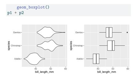
Both plots share the same data (penguins) and the same aesthetic mappings(bill\_length to the x-axis and species to the y-axis). Where they differ is the geometry: the plot on the left uses the violin while the one on the right uses the boxplot.
